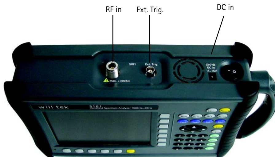
Figure 1 9101 connectors on the top of the instrument
